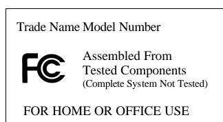
(2) Label text and information should be in a size of type large enough to be readily legible, consistent with the dimensions of the equipment and the label. However, the type size for the text is not required to be larger than eight point.
